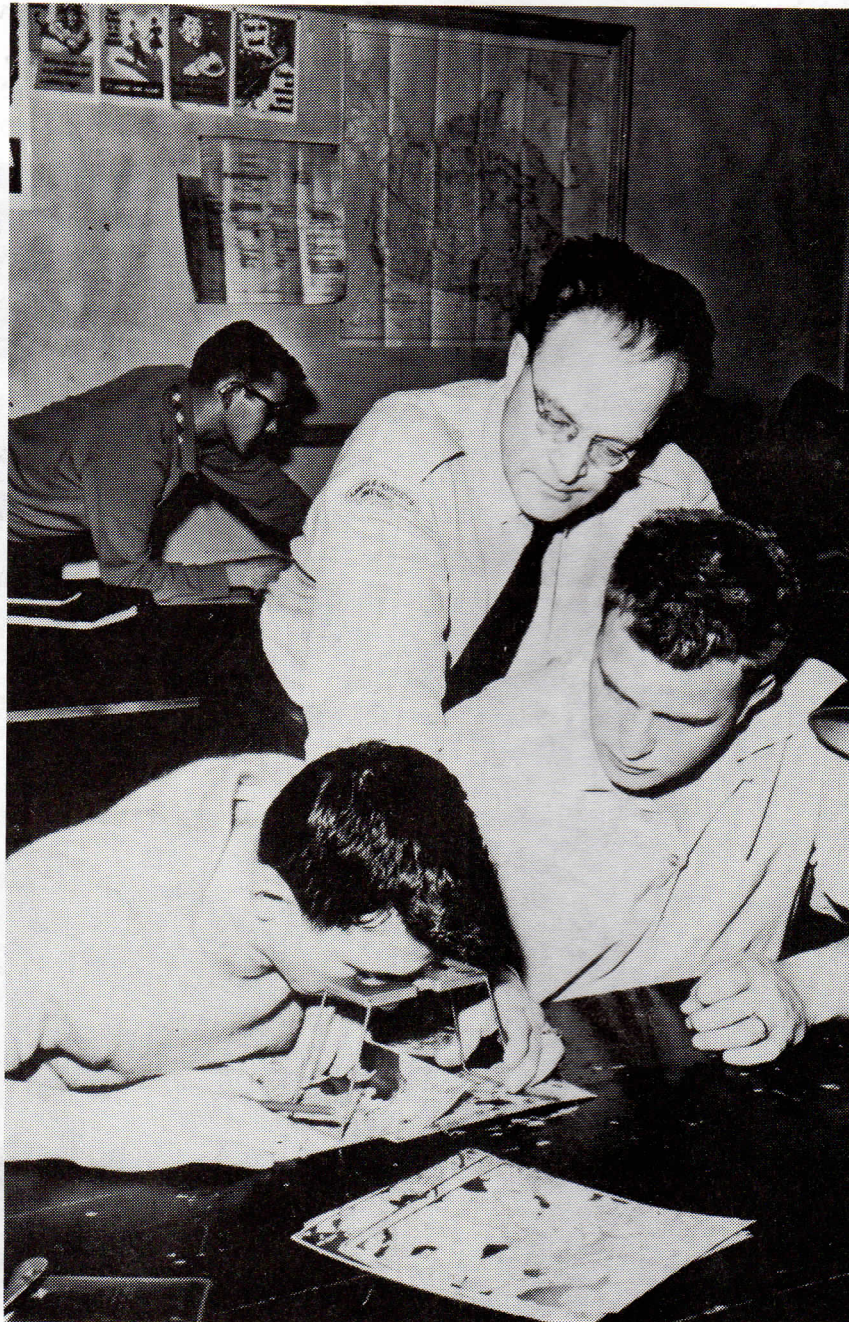
Students at the Forest Ranger School use a stereoscope to interpret the information contained in aerial photographs.
